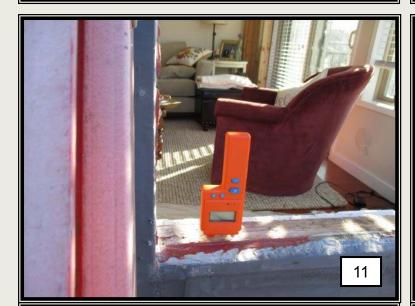
Moisture Meter Readings (MMR's) were gathered from the framing members after the windows removal. All readings were recorded in the normal range.
